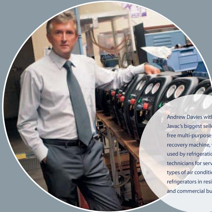
Andrew Davies with one of Javac's biggest sellers, the oil-free multi-purpose refrigerant recovery machine, which is used by refrigeration service technicians for servicing most types of air conditioners and refrigerators in residential and commercial buildings.
